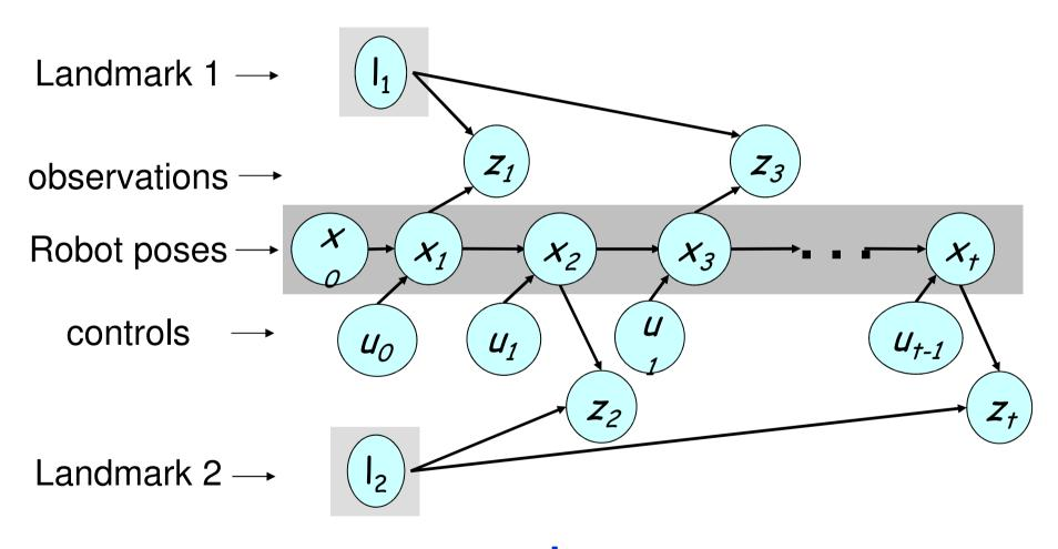
Knowledge of the robot's true path renders landmark positions conditionally independent
