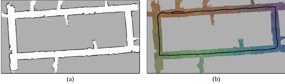
Figure 1: (a) Occupancy grid generated using odometry and a laser range-finder. (b) Combined signal strength map for three beacons, as indicated by the intensity in the red, green and blue color channels. Note that most of the values in this map are interpolated; the heavy line indicates the path of the robot that made the actual measurements.
