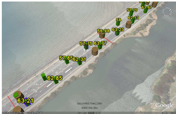
Figure 9: Satellite image of the first experiment site I-80 near Berkeley, CA. The red lines represent the actual locations of the VTLs, the blue squares show the speed recorded by the VTL, the green squares represent the position and speed stored in the phone log. The brown circles represent the speed measurements recorded from the vehicle speedometer.
