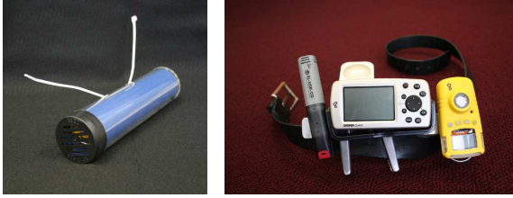
Figure 2: The automotive and personal version of the data-logging sensor platform
