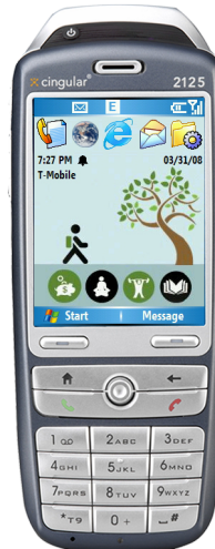
Figure 1 (left) The UbiGreen Transportation Display shows transit behavior as "wallpaper" on a phone's screen. Here the tree is nearly full of leaves, indicating that the user has completed several green trips for the week. (top) The MSP sensor worn near the waist and the phone's GSM cell tower data are used to semi-automatically infer transportation mode.
