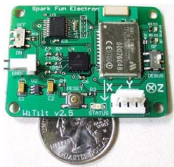
Figure 1. WiTilt Tri-Axial Bluetooth Accelerometer.
