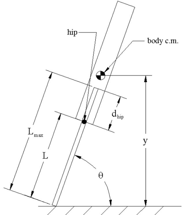
Fig. 2. 2D hopping machine in stance. The body is not shown.
