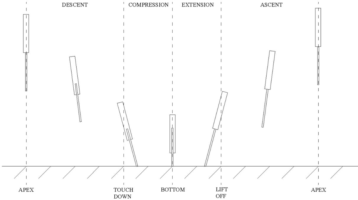
Fig. 1. Phase diagram of a hopping cycle.
