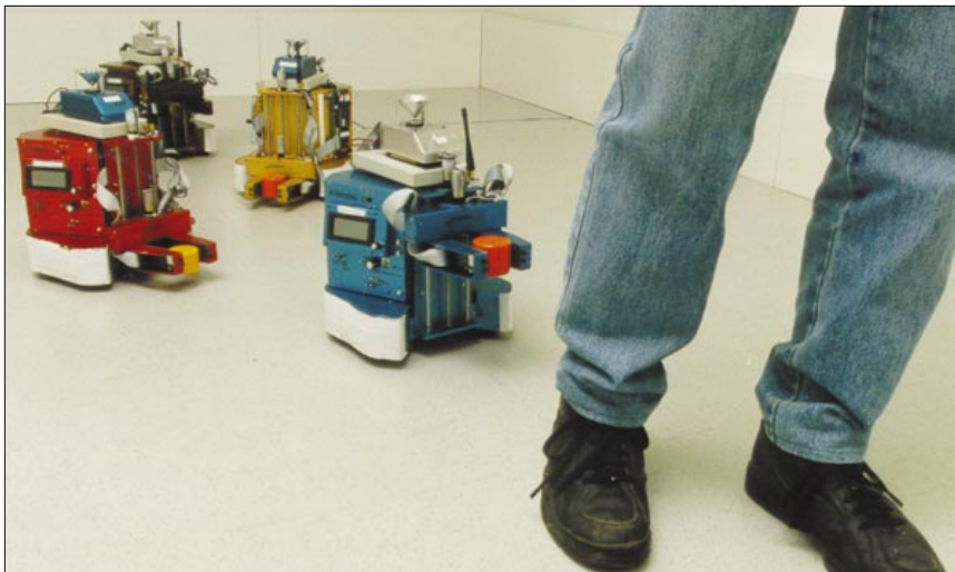
Figure 2. Four IS Robotics R2e mobile robots engaged in collecting pucks and following a human. The robots are equipped with mobile bases, grippers, infrared and tactile sensors, and radios for communication.
