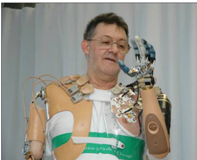
Figure 3. An advanced prosthetic arm with targeted reinnervation-based myoelectric control.
