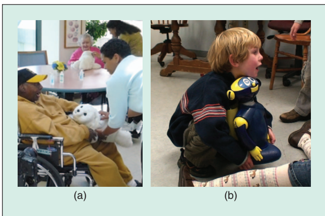
Figure 5. Socially interactive robots for behavioral therapy, personalized care, and wellness/health promotion. (a) Paro, a huggable baby harp seal robot designed for use in hospitals and nursing homes. (b) CosmoBot, a robot designed for play therapy for children with developmental disorders.
