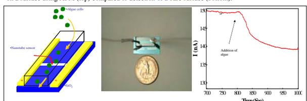
Figure 3: Schematic of carbon nanotube sensor (left) and conductivity profile of sensor following addition of algae (right).
