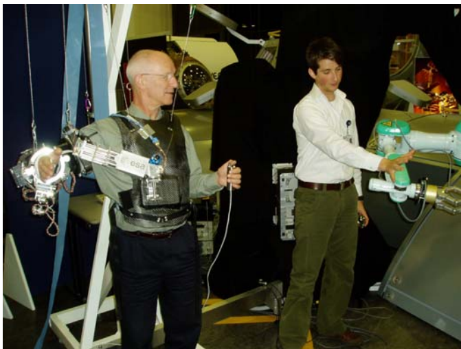
Figure 1: The ESA Human Arm Exoskeleton as worn by ESA astronaut Claude Nicolier during a training session with a teleoperated robot EUROBOT.
