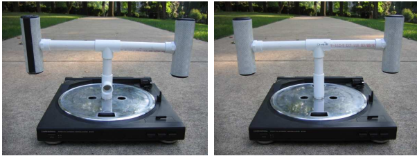
Fig. 5: (Left) Simulated damaged fiducials on the arm’s front side. (Right) Undamaged fiducials on the rear side. This allowed a simultaneous comparison of damaged fiducial position accuracy vs. an undamaged baseline system.
