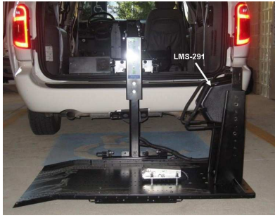
Fig. 2: (Left) Wheelchair lift platform showing LIDAR integration. (Center) Smart wheelchair with retro-reflectors fixed to the front. (Right) Range (top) and reflectivity (bottom) data from a single LIDAR scan. The retro-reflector reflectivity values (two peaks) greatly simplify the feature segmentation process.
