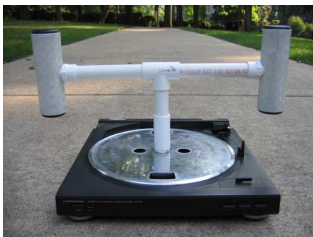
Fig. 3: Test fixture used in fiducial testing. The turntable simulated wheelchair motion, while allowing the estimated wheelchair positions to be projected to a single point.
