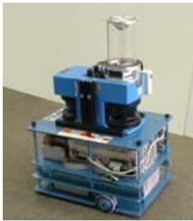
Figure 6: The fully autonomous robot Donald Duck. The panoramic vision system has been mounted right above the wheels. So, for a given position, the fingerprint extraction does not depend on the robot's orientation.
