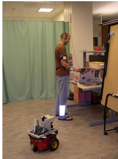
Figure 4: The experimental setup: the participant is performing task 4 (turning pages of a newspaper) with the robot at a social distance. The laser fiducial is on the participant's right leg, the motion sensor on the right arm, and a microphone is worn on standard headphones.
