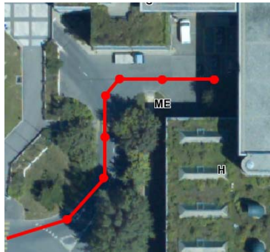
Figure 6.8: The low granularity outdoor topological map superimposed on an architectural sketch of a part of the EPFL campus. This part of the environment represents the zoomed of the rectangle shown in Figure 6.7.
