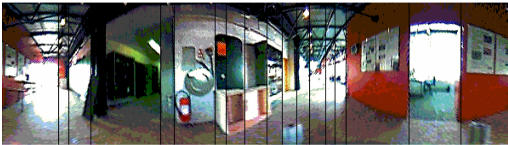
Figure 3.10: The original image with the extracted vertical edges after applying the regrouping filter
