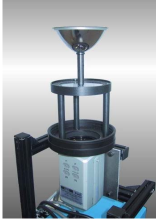
Figure 2.5: Omnidirectional camera system mounted on our mobile platforms (i.e. BIBA robot and "SMART" vehicle)
