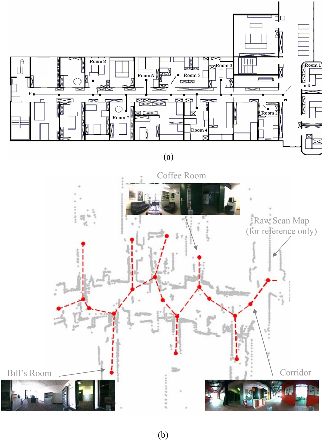
Figure 6.5: (a) Floor plan of the first environment where the experiments have been conducted. The robot starts at the point S and ends at the point E . The trajectory length is 75 m. During this experiment, the robot collected 500 data sets (i.e. images and scans) from the environment. The extracted topological map is superimposed on an architectural sketch of the environment. (b) The extracted topological map given by our method, superimposed on the raw scan map.
