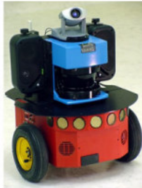
Figure 1: The Pioneer mobile robot base used in the experiments. Shown is the laser (the blue box), camera (mounted on top of the laser), and speakers (mounted on each side of the laser).
