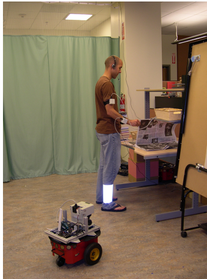
Figure 3: The participant is performing turning pages of a newspaper task with the robot at a social distance. The laser fiducial is on the participant's right leg, the motion capture sensor on the right arm, and a microphone is worn on standard headphones.
